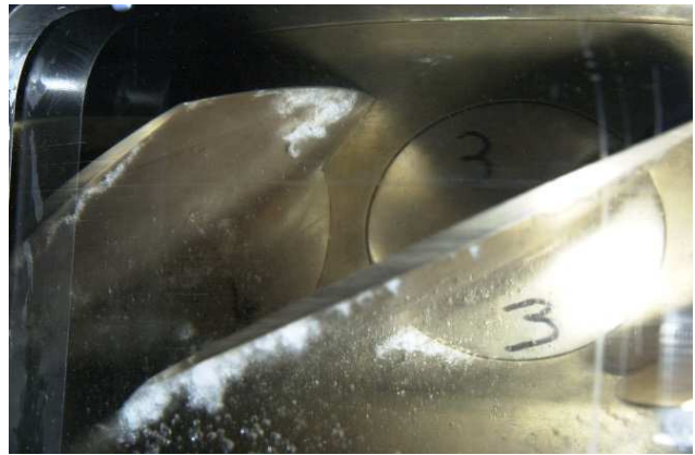
Figure 17 : Cavitation observed on the runner of the Axial turbine, considered as damageable (© Mhylab)
