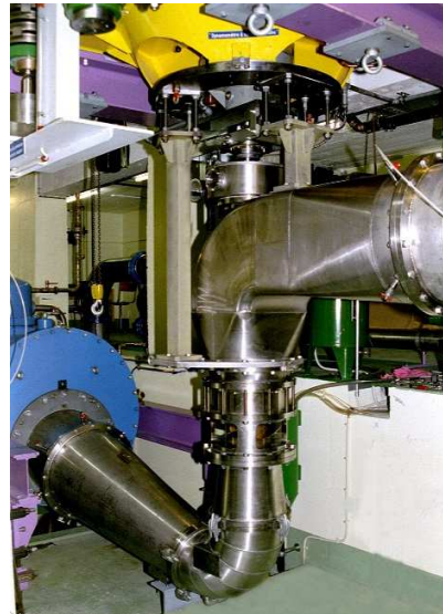
Figure 11 : Scale model of the Axial turbine set on the test bench (© Mhylab)
