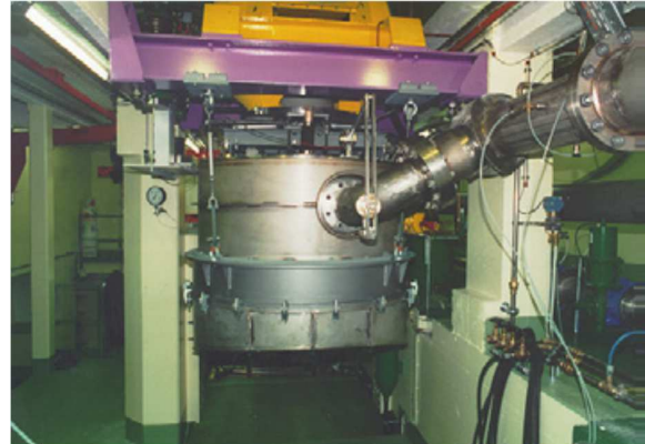
Figure 13 : Scale model of the Pelton turbine set on the test bench (© Mhylab)
