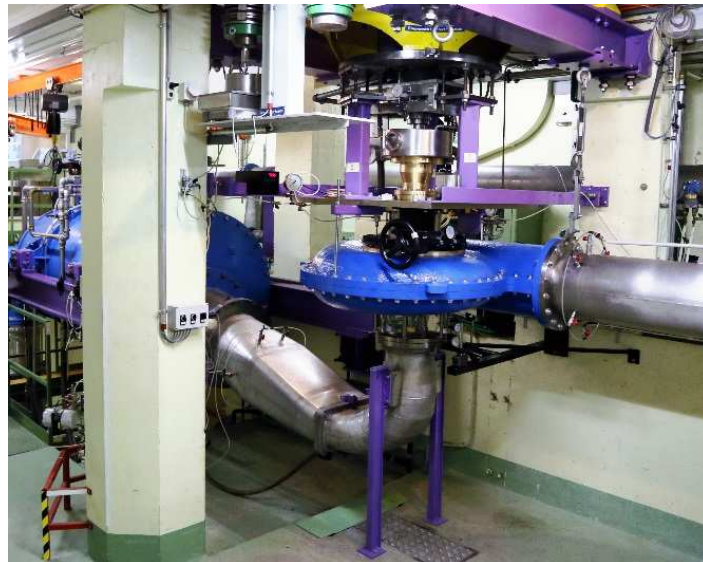
Figure 29 : Scale model of the double-control Diagonal turbine with a spiral casing set on the test bench (© Mhylab)
