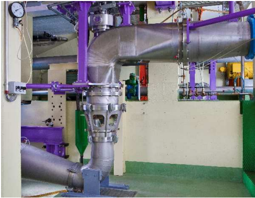
Figure 12 : Scale model of the Diagonal turbine set on the test bench (© Mhylab)
